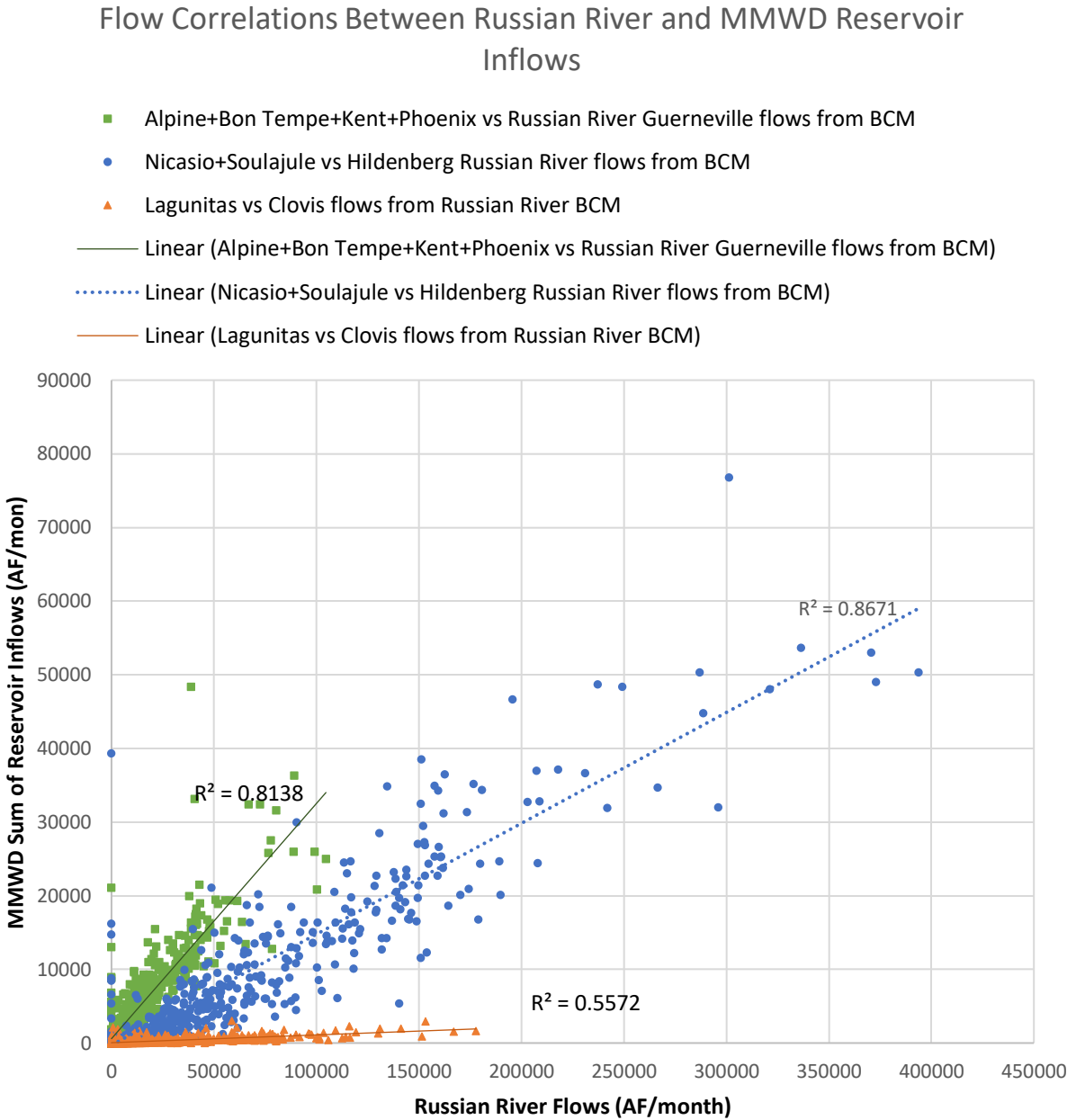
Figure B-6. Monthly correlation of flows between inflows MMWD’s reservoirs versus Russian River BCM flow locations
